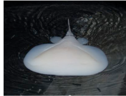
Fig. 8. RayBot experimental prototype in biomimetic body and self-propelled using rack-and-pinion shear actuation of tail.
